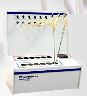
The **Micromeritics FlowPrep O60** applies both heat and a stream of inert gas to the sample. The heat causes contaminants to desorb from the surface and the stream of inert gas sweeps them out of the sample tube. The unit lets you choose the temperature, gas, and flow rate best suited for your sample material and application. Needle valves allow you to introduce the flowing gas slowly to prevent fluidization of samples.
