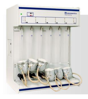
The Micromeritics Smart VacPrep<sup>™</sup> 067 is an advanced six-port system that utilizes vacuum to prepare samples by heating and evacuation. Each of the ports may be operated independently. Samples may be added or removed from degas ports without disturbing the treatment of other samples undergoing preparation. Degassing automatically terminates when the samples have completed all programmed steps.
