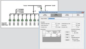
A standard feature of the ASAP 2425 is the integrated twelve-station degas system. Users may prepare up to twelve samples simultaneously. The sample degas procedure is software-controlled and allows easy-to-specify parameters for custom degas and sample preparation. User-defined evacuation rates and temperature ramps are provided to support even the most difficult-to-prepare samples.
